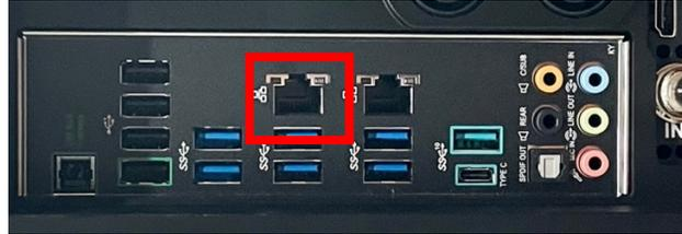
\*\*\* If you received your SurfaceGo+ separate from a system (*or it has shipped after your system has shipped*) you may need to configure the network port manually for use. Please use the following to configure the default network port shown above for use.
